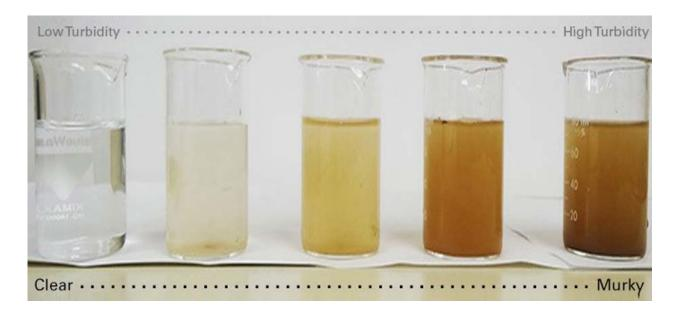
**Turbidity** is defined as the cloudiness or haziness of water caused by large numbers of individual particles that are in water. The measurement of turbidity (in NTUs) is a key test of water quality, and we monitor it because it is a good indicator of the effectiveness of our filtration system. The higher this number is, the cloudier the water will appear. Having an average reading of 0.014 NTU in our filtered water shows that the plant is producing water with exceptional clarity.
