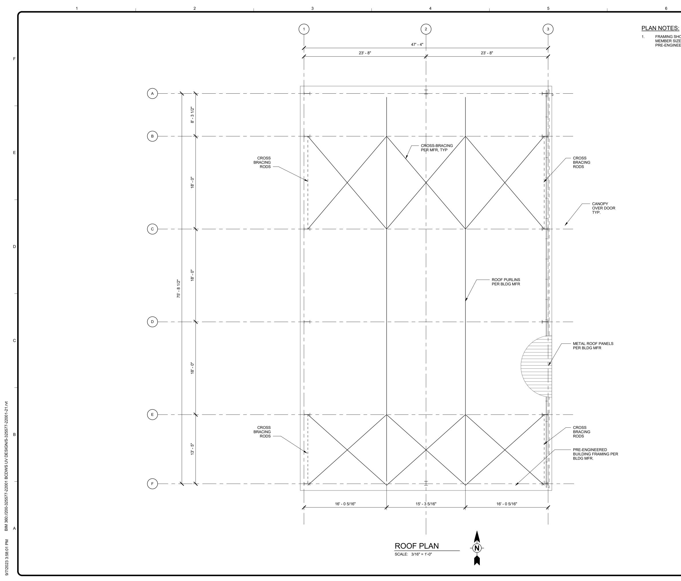
1. FRAMING SHOWN IN THE PLAN IS SCHEMATIC ONLY. ACTUAL FRAMING LAYOUT, MEMBER SIZES, AND CONNECTIONS ARE TO BE DESIGNED AND PROVIDED BY THE PRE-ENGINEERED METAL BUILDING MANUFACTURER
